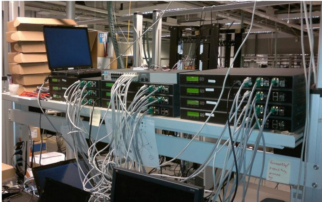
Figure 3. Ten node WMN system set up in the Nokia Siemens Networks Mobile Backhaul Research laboratory
