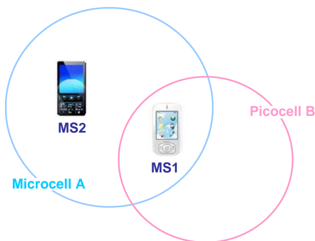
Figure 3-15: Cell selection scenario for a high loaded cell [Amzallag08]
